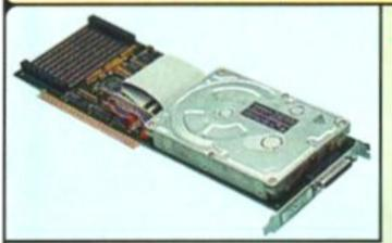
The Impact II HC8 hard cards are the equivalent of the HD8+ hard drive, but for the 1500 and 2000 models. They are some of the fastest hard drives available, and incorporate an unpopulated 8<sub>Mb</sub> RAM expansion.
