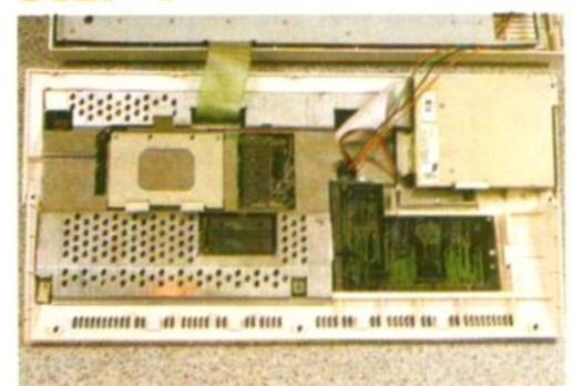
Remove the three screws at the front and the two at the sides of the A1200. This frees the top half of the case. In the A600 you will need to remove the three screws at the front, and the one screw on the right-hand edge. Lift off the top of the case. A600 owners will need to disconnect the cable connecting the keyboard lights, and A1200
