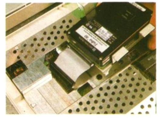
Connect the cable socket to the pins on the motherboard by applying firm pressure until it fits correctly. Make sure that no pins protrude from either side of the plug block, and that none of the pins have been bent by the socket.
