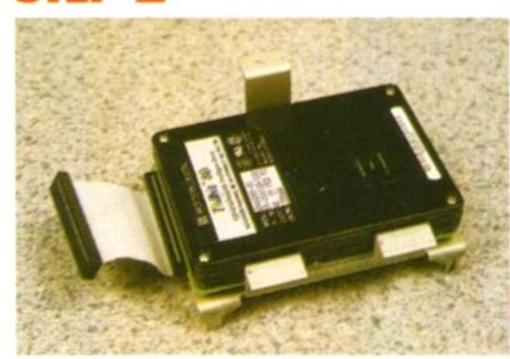
Remove the cradle from the Amiga, and screw the hard disk to it as shown here. It's important that you do get it the right way around.
